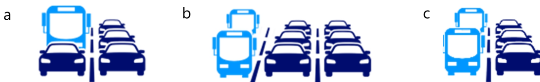
Figure 12. Three DBLs scenarios for the Sioux Falls 2014 road / PT networks, (a) No DBLs; (b) Added; (c) Converted DBLs.
